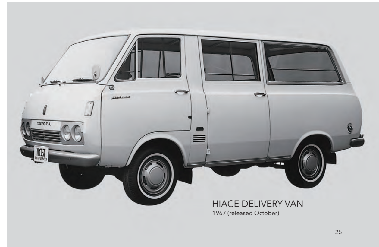
1345cc, 65 horsepower engine, load capacity 500-850kg The HIACE DELIVERY VAN was designed and developed as a genuine all-weather cargo-passenger vehicle. By adopting a monocoque body structure, it made the floor low and enabled securing a wide loading space. Easy to get in and out, easy to load and unload cargo, while having sufficient functionality as a commercial vehicle, it's a new commercial vehicle with a passenger car mood, designed based on the spirit of respect for people. It demonstrated the foresight of TOYOTA's technical team in quickly adopting the van conversion of trucks that was trending worldwide.
