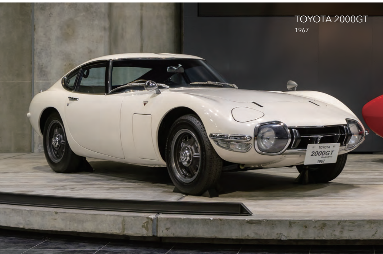
Top speed 220km/h, maximum cruising speed 205km/h, 0-400m in 15.9 seconds A crystallization of advanced technology developed with the cooperation of Yamaha Motor Co., Ltd., possessing world-class top performance in the 2000cc class GT (Grand Touring) while also having luxurious practicality for city driving. In ultra-high-speed endurance trials, it ran at an average speed of 206.18km/h for 78 consecutive hours covering 16,000km, establishing 3 world records and 13 international records. It has an elegant style wrapped in an ideal body with smooth curves that extremely reduced air resistance, determined as a package for fast driving—the position and size of the engine, chassis, interior dimensions, etc. A prototype converted to open-top was used in the movie 007: You Only Live Twice, making its name known worldwide. A car that fused both performance and beauty at the highest level.
